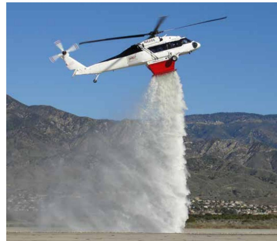
▲ The Helitak FT4500 UH60/S70 Fire Tank dropping 1100 gallons in 4.5 seconds.
